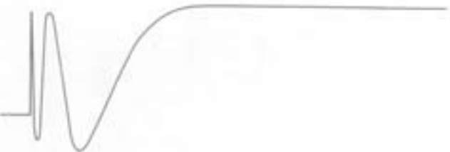
This is the step signal response of a "time-corrected" crossover system. Although time smear is reduced, phase distortions remain unchanged.
