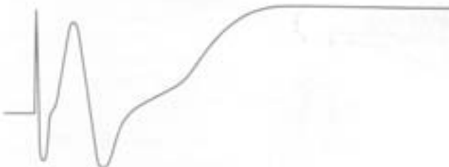
The step signal response of a conventional crossover system illustrates both time smear and phase distortions of a transient signal.
