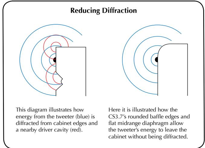
The speaker's front baffle is machined from aluminum, a material more than 30 times as strong as the usual MDF. In addition to reducing unwanted vibrations, aluminum also provides a rigid mounting of the drivers so they cannot move, even a miniscule amount, in recoil from the forces they generate to accelerate the diaphragm (every force has an equal and opposite force).
