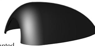
The construction of the cabinet sides also plays its part in the CS3.7's rigid, low vibration cabinet. The sides are made of 15 layers of hardwood laminated together into a curved shape under high pressure. This results in a much stronger panel than usual, with the curves adding greatly to its rigidity. The rounding at the front of the speaker also reduces unwanted diffraction, and the gentle rounding along the cabinet sides creates non-parallel walls to minimize internal resonances.
