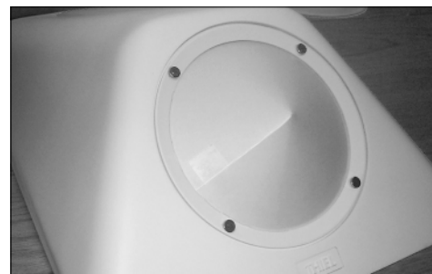
Painting mask installed
